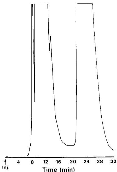
Fig. 1. Chromatogram resulting from preparative HPLC on an extract of an 8- to 16-h urine collection from the volunteer after dosing with Camoquine (600 mg as base). Collection of metabolite II was begun at 21 min and terminated at 28 min.
